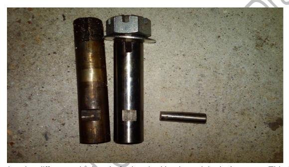
Notice the difference in the shaft slot size/depth....original v/s repro. This is why some pins are mushroomed & outside the axle housing receiver because they do not fit properly as intended.
