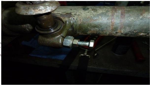
Set up like above with the bolt thread full engaged in the now threaded tapered pin. Then screw the bolt's grade 8 nut in a clockwise, off the bolt direction, while holding the bolt head, if needed.
