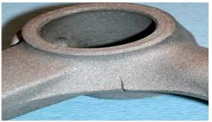
When the bell crank is off check carefully for cracks that they are renowned for, replace as needed. There was an official modification the Australian Army used to rectify the issue. Some welders are better than others I guess.
