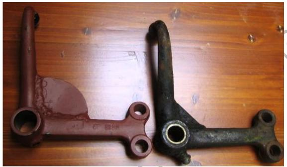
If a worn bell crank shaft needs replacing, they are not easy to remove using the TM method of driving out the tapered [with a flat that engages the flat on the bell crank pin] lock pin toward the left front wheel.
