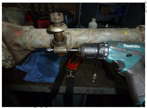
Once the hole is drilled, start tapping the thread.
