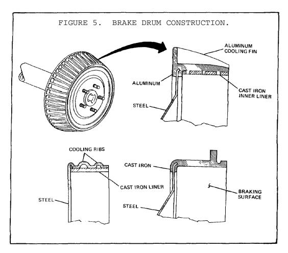
The brake drums are usually made of pressed steel, cast iron, or a combination of the two metals. Cast-iron drums dissipate the heat produced by friction more rapidly than steel drums and have better friction surfaces. However, if a cast-iron drum is made as strong as it should be, it will be much heavier than a steel drum.
