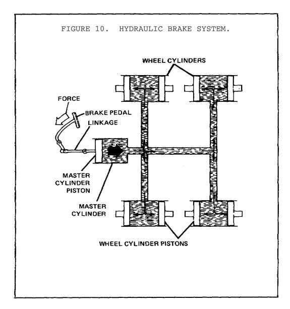
In hydraulic braking systems, the pressure applied at the brake pedal is transmitted to the brake mechanism by a liquid. Since a liquid cannot be compressed under ordinary pressures, force is transmitted solidly just as if rods were used. Force exerted at any point upon a confined liquid is distributed equally through the liquid in all directions so that all brakes are applied equally.
