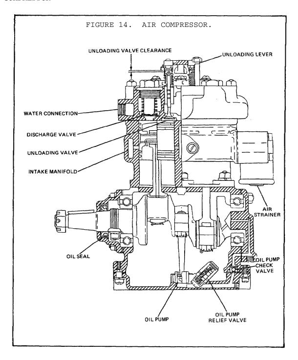
The air compressor pumps up the air pressure needed to operate the air-hydraulic cylinder. The compressor is driven by the vehicle's engine and turns all the time the engine is running.
