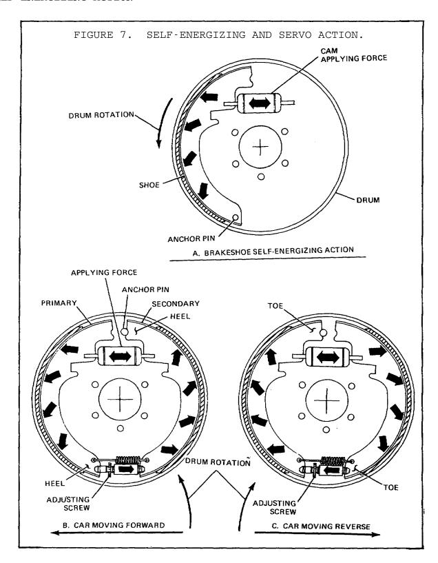
The brake operating linkage alone does not provide enough mechanical advantage for good braking. Some way of increasing the pressure of the brake shoes is needed. A self-energizing action can be used to do this, once the setting of the shoes is started by the movement of the linkage. There are several variations of this self-energizing action, but it is always done by the shoes themselves as they tend to turn with the turning drum.
