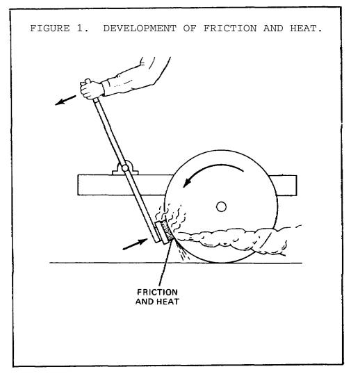
Brakes on early motor vehicles were nothing more than modified wagon brakes used on horse-drawn wagons. These were a hand-operated, mechanical, lever-type brakes that forced a piece of wood against one or more of the wheels. This caused friction or a drag on the wheel or wheels.
