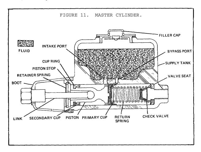
The master cylinder housing is an iron casting which contains the cylinder and a large reservoir for the brake fluid. The reservoir carries enough reserve fluid to ensure proper operation of the braking system. It is filled through a hole at the top which is sealed by a removable filler cap containing a vent. The cylinder is connected to the reservoir by two drilled holes or ports, a large intake port, and a small bypass port.
