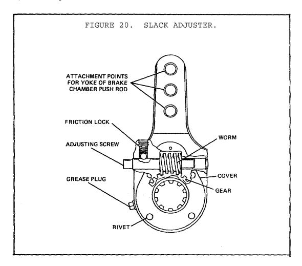
The pushrod of the brake chamber is connected to a slack adjuster. The slack adjuster serves two purposes: to change the back and forth motion of the pushrod to rotary motion and to make minor adjustments to the brake shoes and linings.
