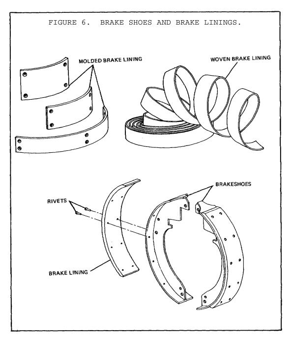
Brake shoes are made of malleable iron, cast steel, drop-forged steel, pressed steel, or cast aluminum. Pressed steel is usually used because it is cheaper to produce in large quantities. Steel shoes expand at approximately the same rate as the drum when heat is produced by brake application, thereby maintaining the clearance between the brake drum and the brake shoe under most conditions.
