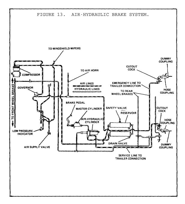
An air-hydraulic brake system has all the components of a straight hydraulic system plus those of the compressed air system. Besides boosting the hydraulic pressure of the brakes on the truck, the compressed air system can also be used to apply the brakes of a trailer and operate accessories such as the wiper motor and horn.
