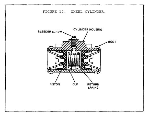
The wheel cylinder changes hydraulic pressure into mechanical force that pushes the brake shoes against the drum. The wheel cylinder housing is mounted on the brake backing plate. Inside the cylinder are two pistons which are moved in opposite directions by hydraulic pressure and which, at the same time, push the shoes against the drum. The piston or piston stems are connected directly to the shoes. Rubber piston cups fit in the
