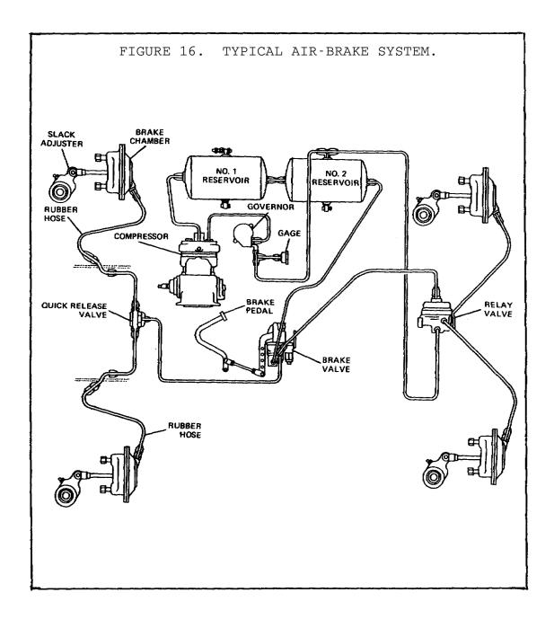
The compressed air system, consisting of the air compressor, governor, and two reservoirs, is about the same as the one we studied for air-hydraulic brake systems. There may be some minor differences in the air compressor and governor, but they will not affect the maintenance practices on the components.
