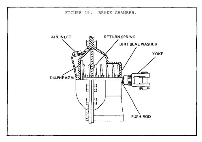
The brake chambers at each wheel convert air pressure to mechanical motion. When air enters the air inlet, it moves the diaphragm which moves the pushrod.
