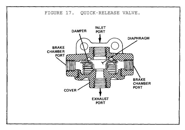
The air line from the brake valve to the front axle goes to a component known as a quick-release valve. When the brakes are applied, the quick-release valve directs compressed air to the right and left front brake chambers. When the pedal is released, the air from the brake chambers escapes out of the quick-release valve and releases the front brakes. The air in the line from the brake valve escapes through the exhaust valve in the brake valve.
