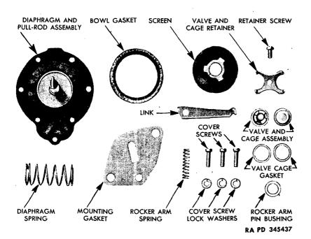
Figure 4—Typical Repair Kit Contents
