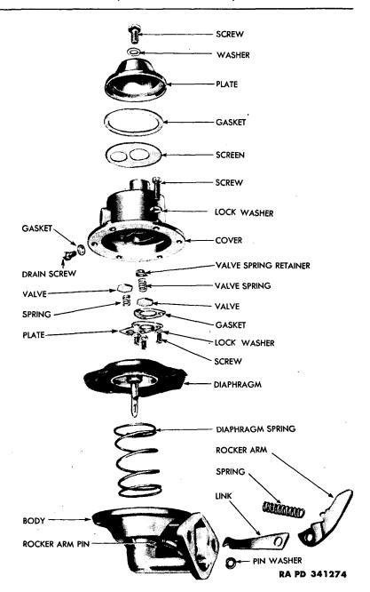
Figure 14—Fuel Pump—Disassembled (Typical Series R Construction)
