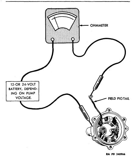
Figure 53—Testing Field Coil With Ohmmeter
