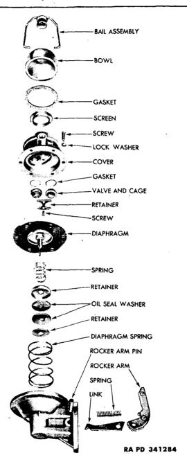
Figure 24—Fuel Pump—Disassembled (Typical Series AF Construction)
