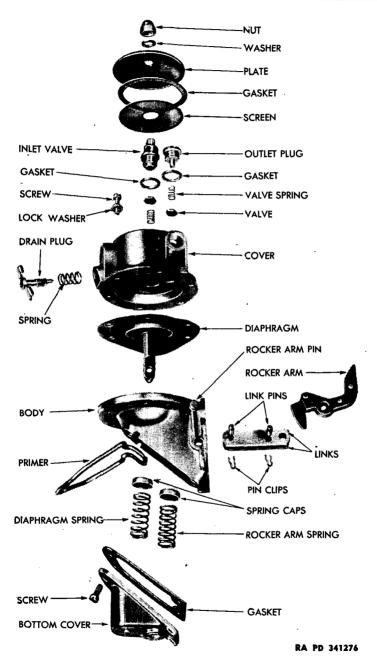
Figure 16—Fuel Pump—Disassembled (Typical Series S Construction)
