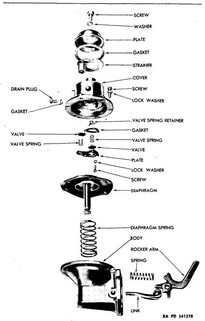
Figure 18—Fuel Pump—Disassembled (Typical Series T Construction)
