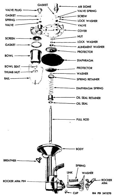
Figure 10—Fuel Pump—Disassembled (Typical Series IHC Special Construction)
