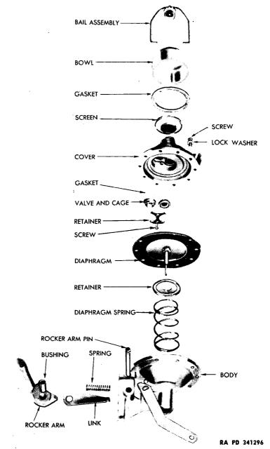
Figure 36—Fuel Pump—Disassembled (Typical Series AU Construction)
