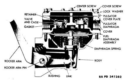
Figure 2—Fuel Pump, Series BF—Sectional View
