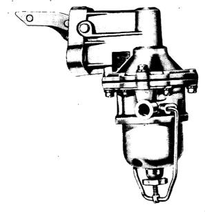
Figure 33—Fuel Pump, Series AT
