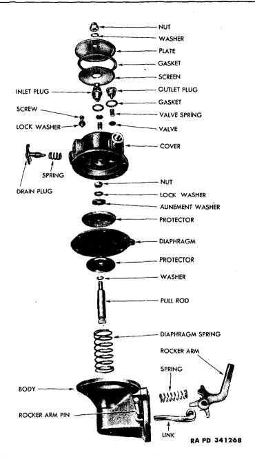
Figure 8—Fuel Pump—Disassembled (Typical Series G Construction)
