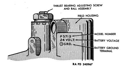
Figure 48—Voltage and Polatity Identification
