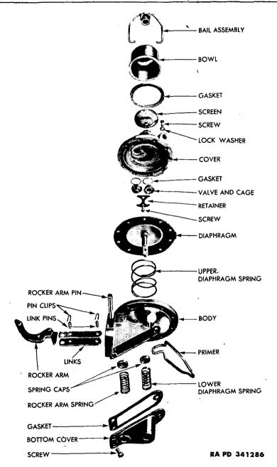
Figure 26—Fuel Pump—Disassembled (Typical Series AG Construction)
