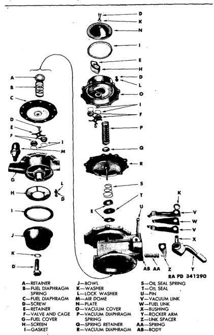
Figure 30—Fuel and Vacuum Pump—Disassembled (Typical Series AJ and AV Construction)
