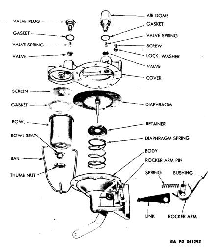
Figure 32—Fuel Pump—Disassembled (Typical Series AK
