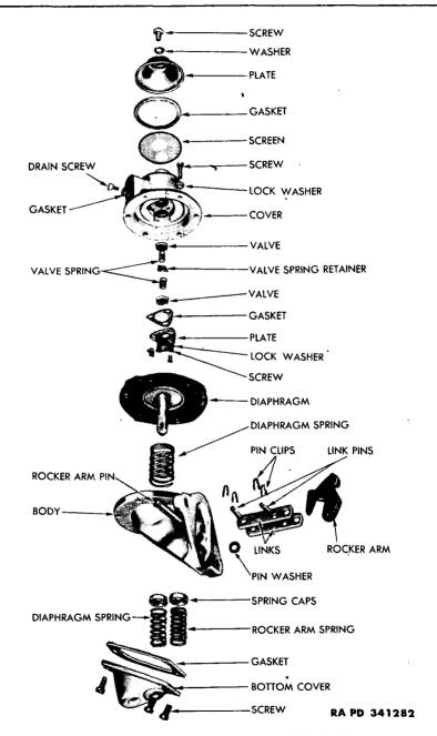
Figure 22—Fuel Pump—Disassembled (Typical Series AC Construction)
