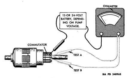
Figure 54—Testing Armature
