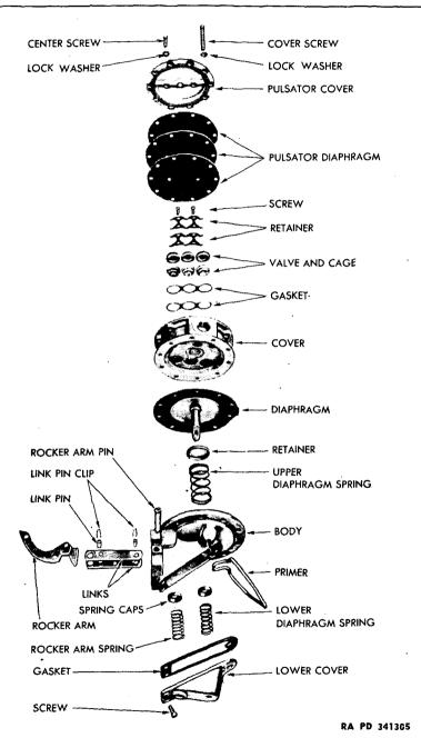
Figure 45—Fuel Pump—Disassembled (Typical Series BH Construction)
