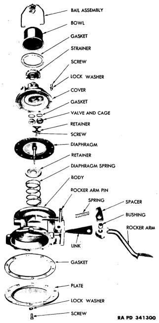
Figure 40—Fuel Pump—Disassembled (Typical Series BE Construction)
