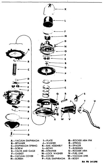
Figure 38—Fuel and Vacuum Pump—Disassembled (Typical Series AX Construction)
