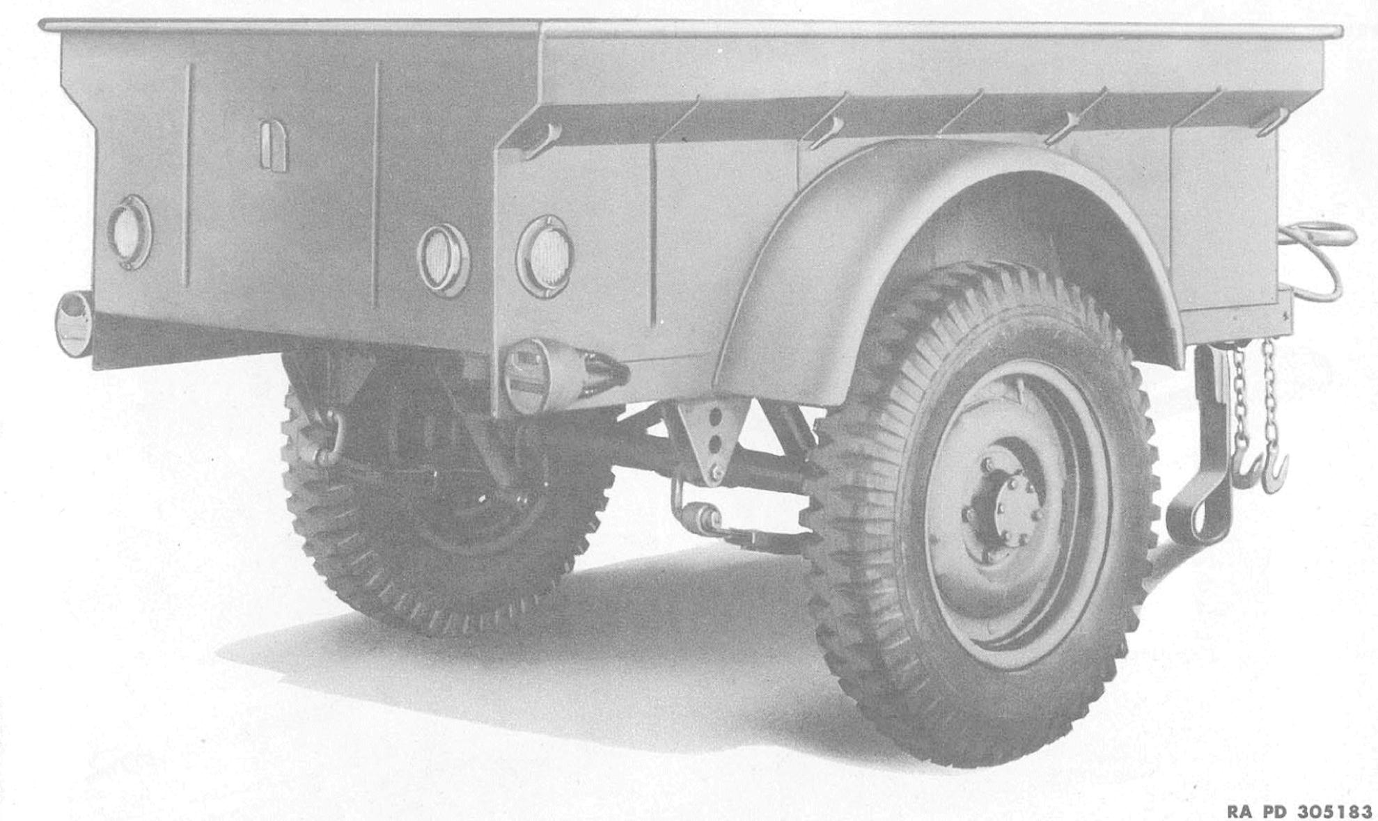
FIGURE A—TRAILER, ¼-TON PAYLOAD, 2-WHEEL, CARGO, 1942-43, AMERICAN BANTAM T-3
