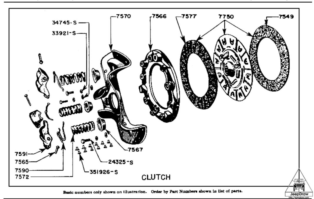
Clutch Disc 0201 GPW 7549 Pacing - clutch disc 371.567 1 751926-S Rivet -clutch feeling 374631 Dine anny-clutch 4.65 636755 GPW 7550 Hub-clutch release bearing 639651 GPW 7561 ī Spring-dutch release bearing 630117 GPV 7962
